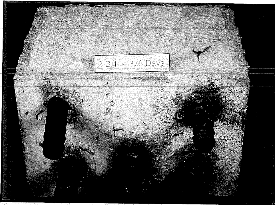
(a) Specimen 2 B.1, One year of Exposure
