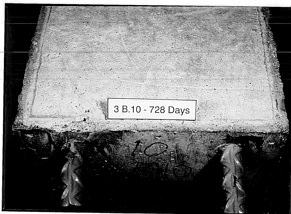
(b) Specimen 3 B.10, Two Years of Exposure
