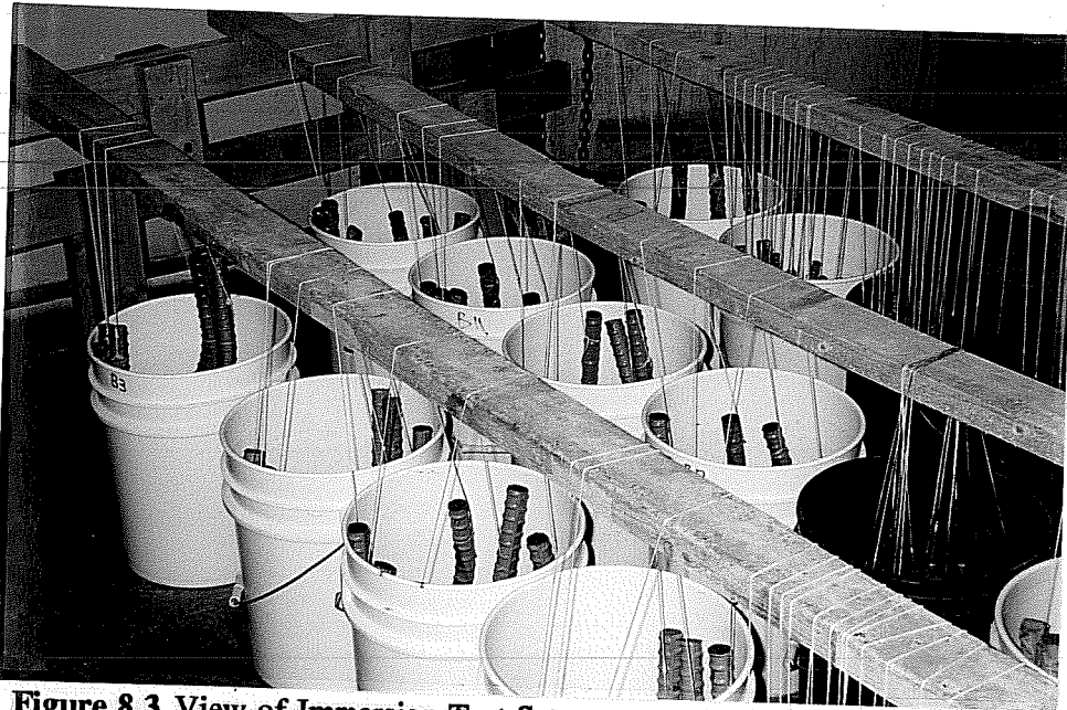
Figure 8.3 View of Immersion Test Setup.
