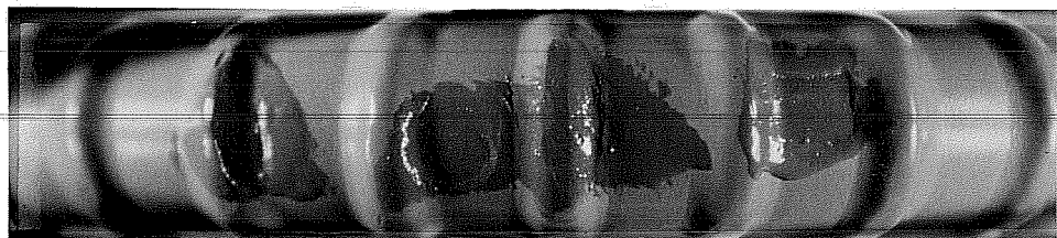
(a) Damage Spots > 6 \times 6 mm, Bar with Parallel Deformations
