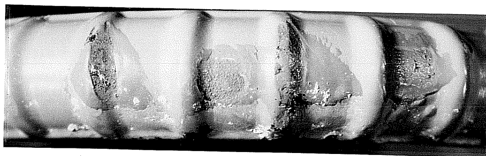
(b) Rust Spotting on Specimen 1 B.2
