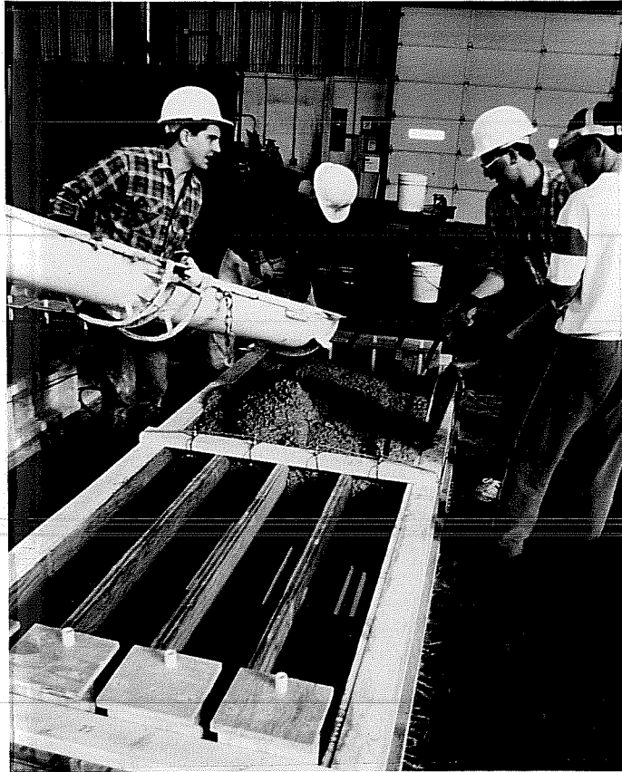
Figure D.13 Casting Beam Specimens.
