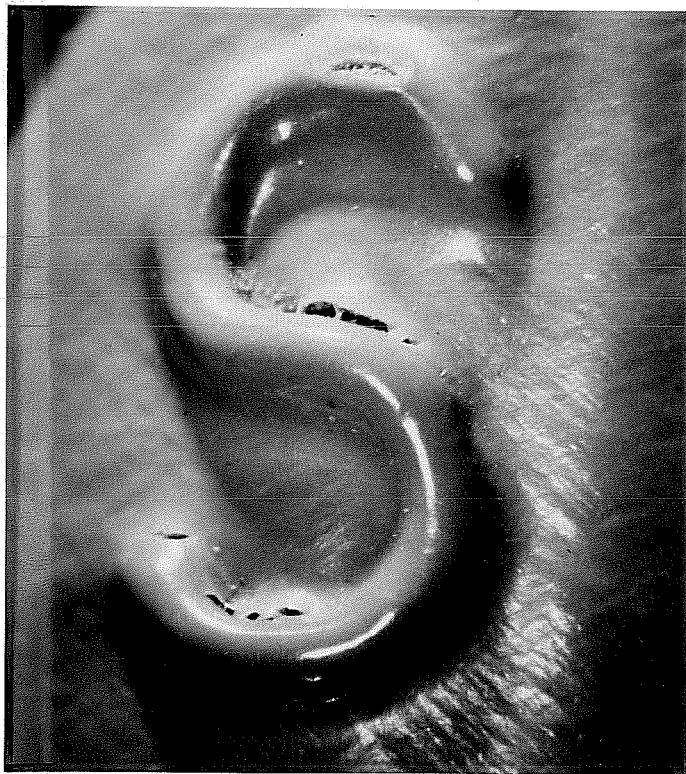
Figure 3.8 Typical Pinholes at Mill Marks on Bar Surface.
